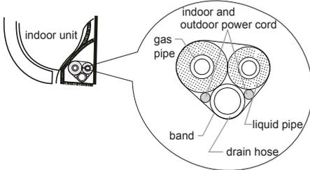
2. Plan for bends in line set and ensure that cable and drain have extra length in those areas. Otherwise route these separate from liquid and gas pipe.
