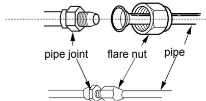
3. Adjust the torque force by referring to the following sheet. Place the open-end wrench on the pipe joint and place the torque wrench on the flare nut. Tighten the flare nut with torque wrench.
