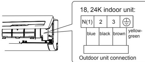
4. Put wiring cover back and then tighten the screw.
