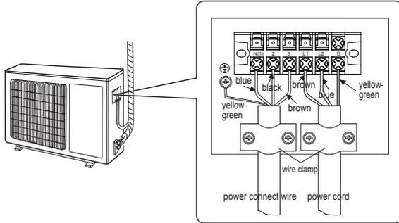
2. Secure the power connection wire and signal control wire with wire clip (only for cooling and heating unit).
