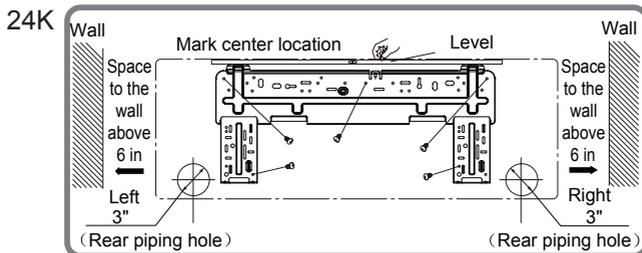
2. Drill hole through wall with a diameter of 3" on the selected location. In order to drain smoothly, slant the hole on the wall slightly downward to the outdoor side with the gradient of 5-10°.
